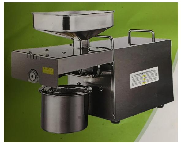
Figure 2. The oil press used for extraction of oil from the cleaned dried black sesame seed.
